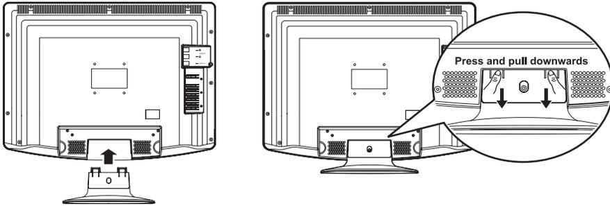
3. To install the base stand, place the base stand on the mounting slot, push the stand till it locks.
