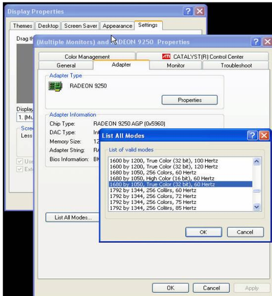
Note: If your video/ graphic card does not support the resolution of 1680 x 1050, then you can try to set the resolution to 1280 x 960 or 1280 x 768 to avoid picture stretching.
