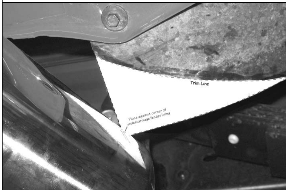
Figure 7 Placement of template on Passenger side rear undercarriage lining.
