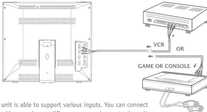
1. This unit is able to support various inputs. You can connect your video recoder, amplifier, game console etc, to the unit.
