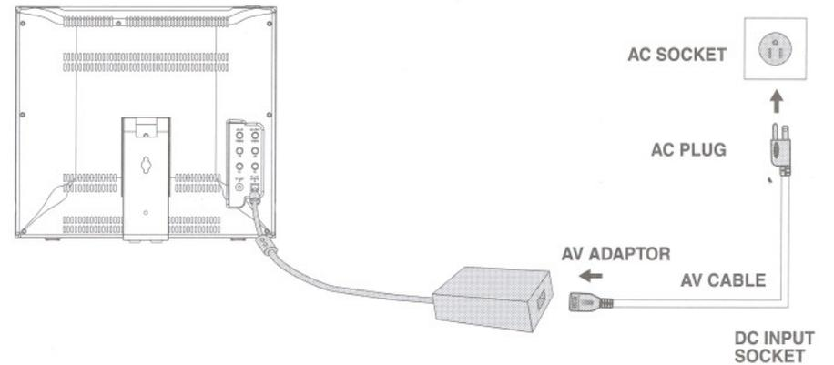
ATTENTION: Ensure the power supply is connected to the unit. When not using unit for a long period of time, remove power adaptor socket from the main power point.
