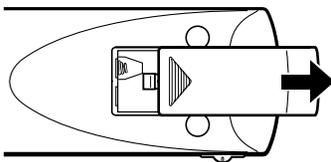
2. Install two “AA” size alkaline batteries. Match the + and - signs on the batteries to the signs on the battery compartment.
