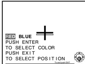
5. Press ▲ (up), ▼ (down), ◀ (left), or ▶ (right) to converge the red or blue line into the green line. When color convergence is correctly adjusted, you will see two single white lines.
