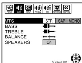
You should leave your TV set to STR so you can automatically receive stereo or monaural sound, depending on the broadcast type. If the stereo sound is noisy, select MONO to reduce the noise. The word STR or SAP is displayed in yellow when the TV receives the signal, and in purple when you have selected the feature.
