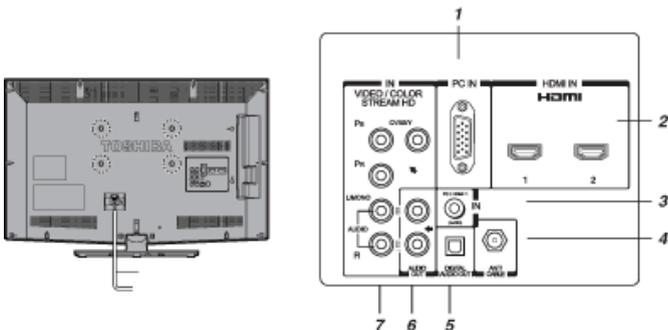
(Sample Illustration) L4200U Series back panel connections
