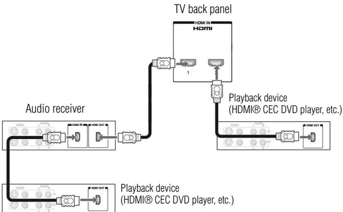
*(Sample Illustration) L4200U Series—HDMI® CEC compatible audio receiver and playback device connections*
