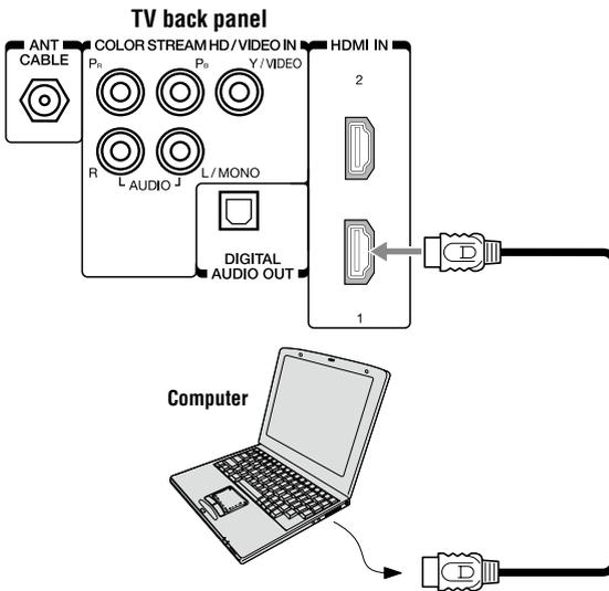
*(Sample Illustration) 32/40/50L1400U Series - Connecting a computer to the TV through the HDMI® terminal.*
