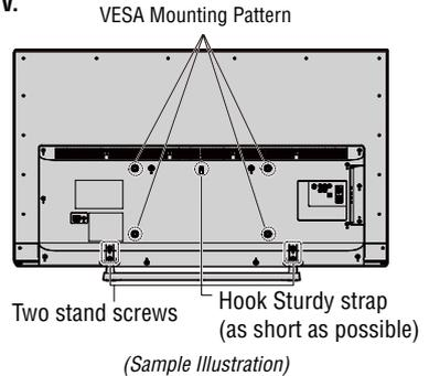
**CAUTION:** Always place the TV on the floor or a sturdy, level, stable surface that can support the weight of the unit. To secure the TV, use a sturdy strap from the hook(s) on the rear of the TV to a wall stud, pillar, or other immovable structure. Make sure the strap is tight, secure, and parallel to the floor.
