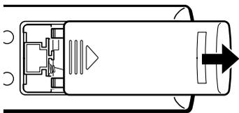
2. Install two “AA” size alkaline batteries. Match the + and – signs on the batteries to the signs on the battery compartment.
