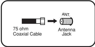
For basic cable service not requiring a Converter/Descrambler box, connect the CATV 75 ohm Coaxial Cable directly to the Antenna Jack on the back of the TV/VCR.
