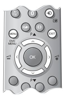
Most video recorders and decoders send a signal through the Scart lead to switch the TV to the correct *Input* socket. Alternatively press the external source selection button - repeatedly until you see the picture from your equipment. You must use this button to view equipment connected using the COMPONENT VIDEO INPUT (**EXT 4**).
