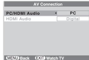
**PC:** Mutes the sound from the HDMI device, and outputs the sound from the PC
