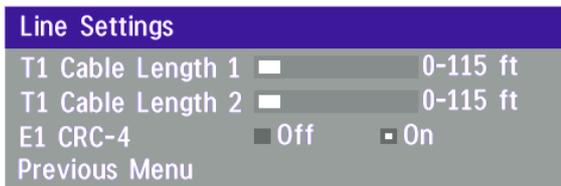
'T1 Cable Length 1' specifies the distance to the CSU connected to the 'E1/T1 1' port on codec 1. Cable Length 2 specifies the cascading distance from the 'E1/T1 2' port on codec 1 to the 'E1/T1 1' port on codec 2. Possible values are 0-115 feet, 80-215 feet, 180-310 feet, 280-410 feet, 375-510 feet, 475-605 feet, 575-690 feet.
