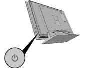
**5.** Switch the TV on by pressing the on/off button on the right side.
