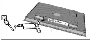
Connect the female plug to the AC socket on AC adaptor.
