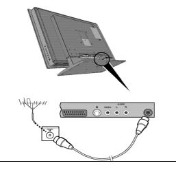
**4.** Connect the outside aerial or cable network to the socket at the back of the TV set.
