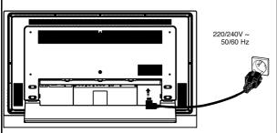
I. Connect the female plug to AC power input of the set.
