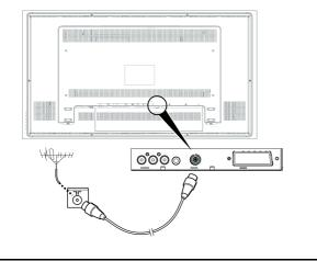
**3.** Connect the outside aerial or cable network to the socket at the back of the TV set.
