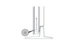
**4.** Switch the TV on by pressing the on/off button on the right side.
