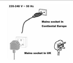
Equipment for the UK is supplied with a mains cable fitted with a moulded plug.
