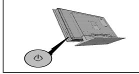
**4.** Switch the TV on by pressing the on/off button on the right side.
