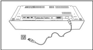
I. Connect the female plug to AC power input of the set.
