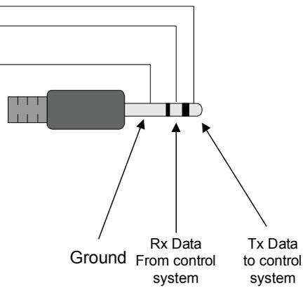
Com Specs: 9600 baud 8 data, 1 stop, no parity
