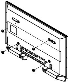
4 Remove the Safety Pins. Fasten the 4 plastic latches assembled at step (3) on the back side of the PDP using the guide holes of the wall mount, push (1) and hook (2) down to secure the PDP on the wall mount as illustrated. Secure the PDP by inserting the Safety Pins.
