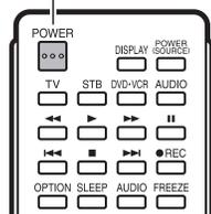
Press **POWER** on the TV or on the remote control unit to turn the power on.
