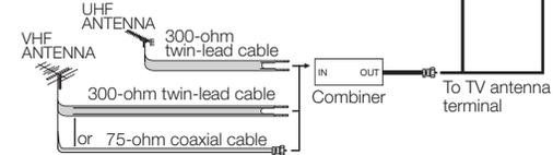
1. A 75-ohm system is generally a round cable with F-type connector that can easily be attached to a terminal without tools.
