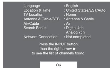
When no channel is received after "Antenna & Cable" was selected in step 6 and a search was carried out.
