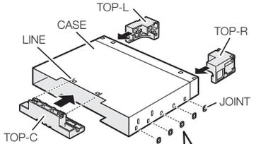
Attach the joints and close the case.
