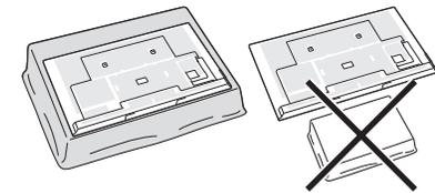
• In the installation procedure, be careful not to catch your fingers between the TV set and the floor.
