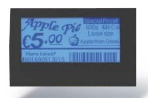
This LCD utilizes memory display elements that require no power except when changing the display content. It is ideal for price tags in supermarkets, etc., where the information displayed does not change for a period of time. The display can easily be changed with a personal computer for efficient management and color variation. This is truly an "electronic paper" that eliminates the need for rewriting or replacement. This new LCD promises a wide range of applications considering its solution.
