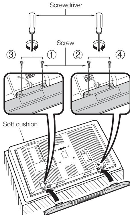
Insert and tighten the 4 screws with the hex key (supplied with the product) in the order of ①, ②, ③ and ④.
