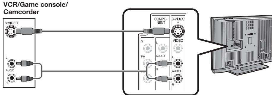
**When using composite cable (commercially available).**
