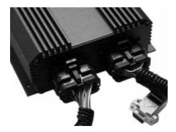
To remove a connector once it is installed, insert a small flat blade screwdriver under the locking clip. Lift the clip while pulling on the connector (never pull on the wires).
