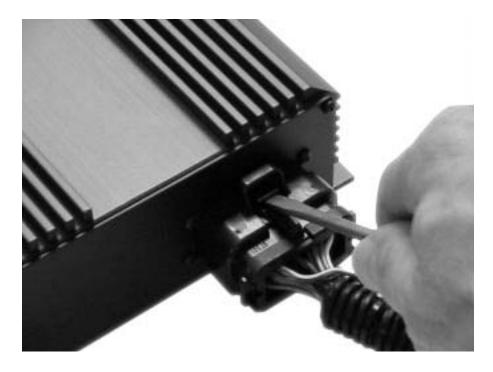
To make installation as easy as possible, the wiring harness provided is completely assembled with connectors that mate to the supplied sensors. Each sensor is connected to the QwikData unit by simply mating the appropriate connectors. (Refer to the QwikData Reference Manual on the CD ROM for a description of the wiring harness and the sensor connections.)
