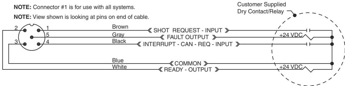
**FIG. 32: External Control Interface Electrical Diagram**
