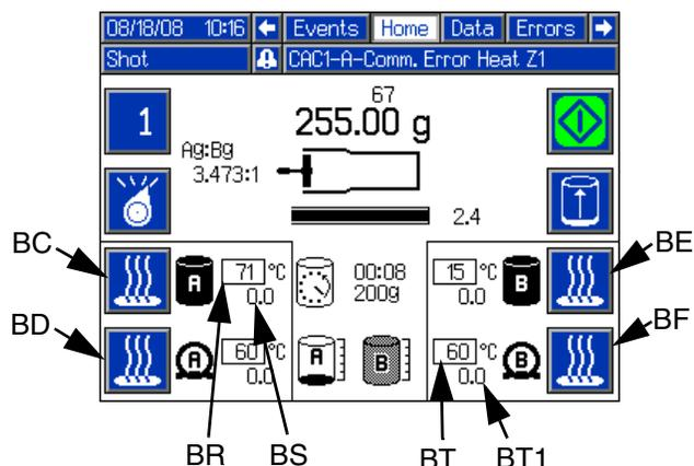
The Tank Fluid Temperature Setpoint (BR), Tank Fluid Temperature (BS), Hose Heater Temperature (BT1), and Hose Heater Temperature Setpoint (BT) display the status of each of the options. To turn the Tank Blanket Heaters or Hose Heaters on or off, press the Tank or Hose Heater On/Off button (BC, BD, BE, BF). See **Heat Options, Screen #2** on page 28 for more information on temperature control setup.
