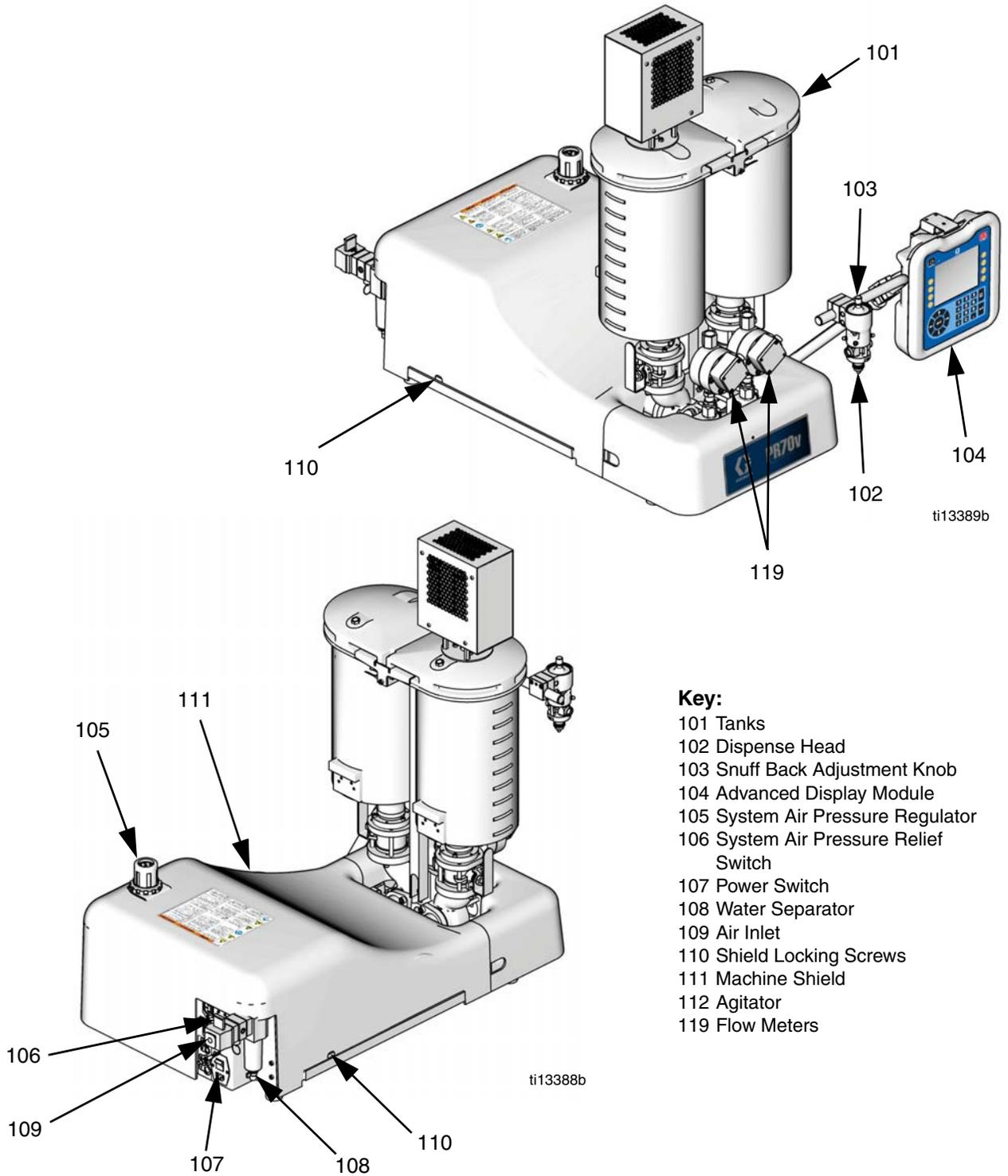
**FIG. 1:PR70v with On-Board Tanks and Other Options**
