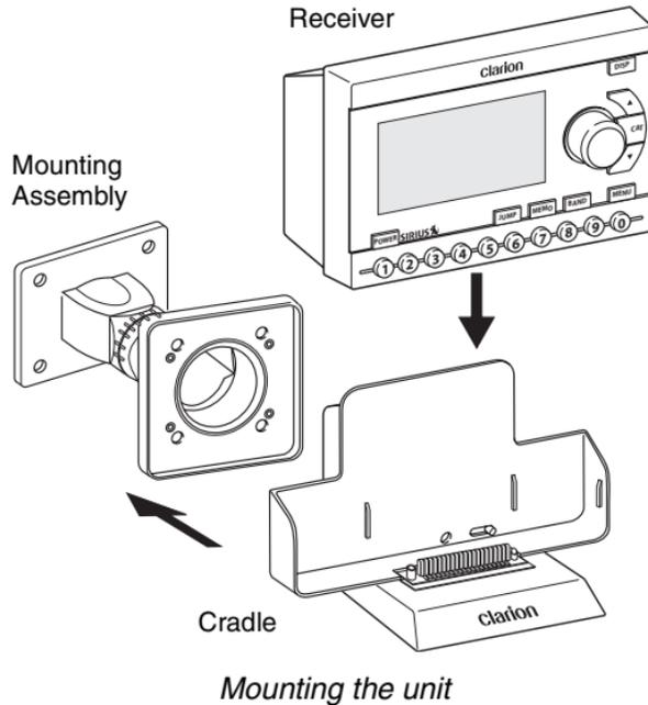
1. Mount the mounting assembly in the vehicle.
