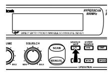
To clear a single frequency from skip memory so the scanner can stop on it during a limit or direct search, press LIMIT to hold the search, press D or — to select the skipped frequency, then press L/O/SEARCH SKIP until LOCKOUT disappears from the display.
