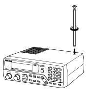
The antenna's length controls its sensitivity. Adjust the length of the telescoping antenna as follows for the best reception.
