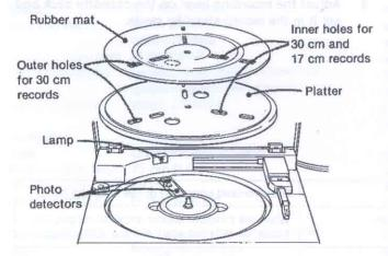
When a 30 cm record is to be played, both inner and outer holes are covered so no beam is transmitted to the photo detectors.
