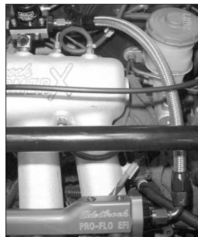
Figure 7 - Fuel Rail to Regulator Line
