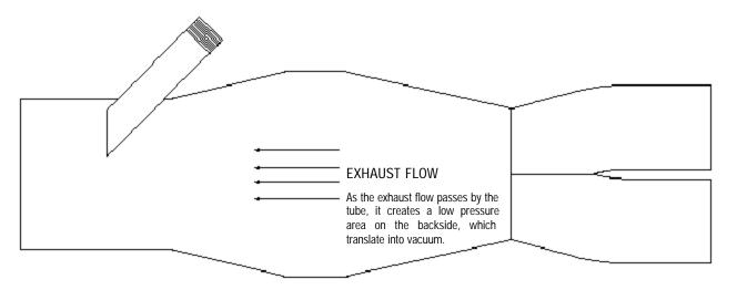
Note: Your Edelbrock Victor Series Race Headers include stainless steel evacuation tubes, O2 sensor bungs and collector mounting tabs to be installed, if needed. Collector mounting tabs should be installed after primary tube tuning has been completed. Evacuation tubes can be positioned on the collector where desired for best fit and hose routing. See the above diagram for recommended installation.
