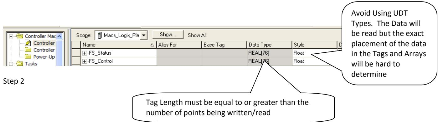
Note that providing dedicated (long), flat structured (not UDT) tags for communications interface to the FieldServer is preferable to polling single length tags in the PLC as it allows for much more efficient communications and reduces complexity when mapping data in the FieldServer. It is better to think of these tags as a "I/O Buffer" Interface that the real tags in the PLC get mapped to.
