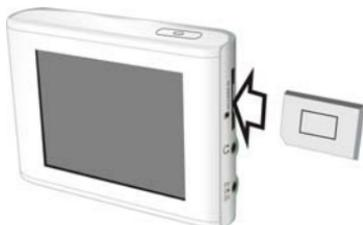
To remove the card, gently press the card in with your fingernail. The card unlocks and protrudes slightly. Then remove the card.
