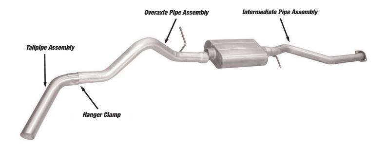
**WARNING:** Support your vehicle with proper jackstands or ramps rated for the total vehicle weight. Place stands so that the rear axle is allowed to hang free for easy system removal.
