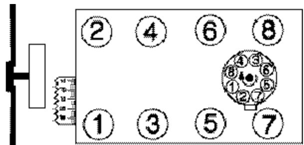
Figure 2 - 262-400 c.i.d. Small Block Chevy Firing Order
