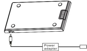
1. Connect the power cord to the battery pack.
