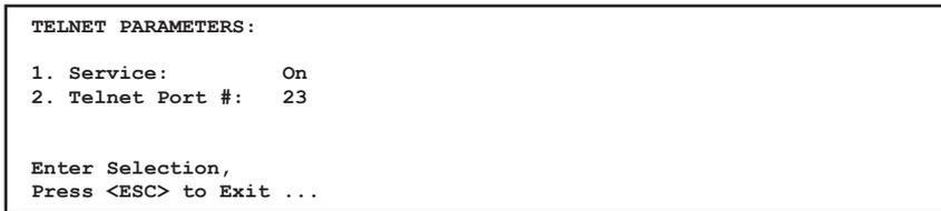
Figure 5.13: Telnet Parameters Menu - Text Interface
