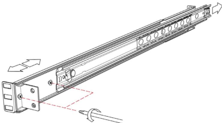
2. Install the rail into the rack by attaching them to the front/rear posts using the appropriate screws and nuts for your rack (not included):
