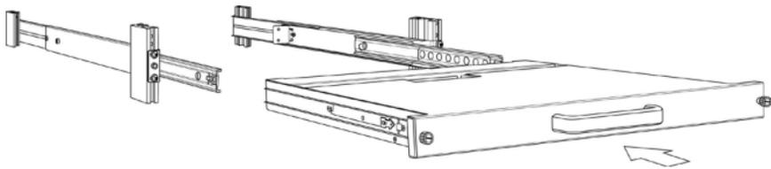
6. Install two screws on each side of the rear console:
