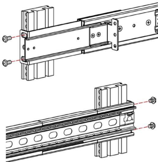
3. Tighten the rear screws that were loosened in Step 1:
