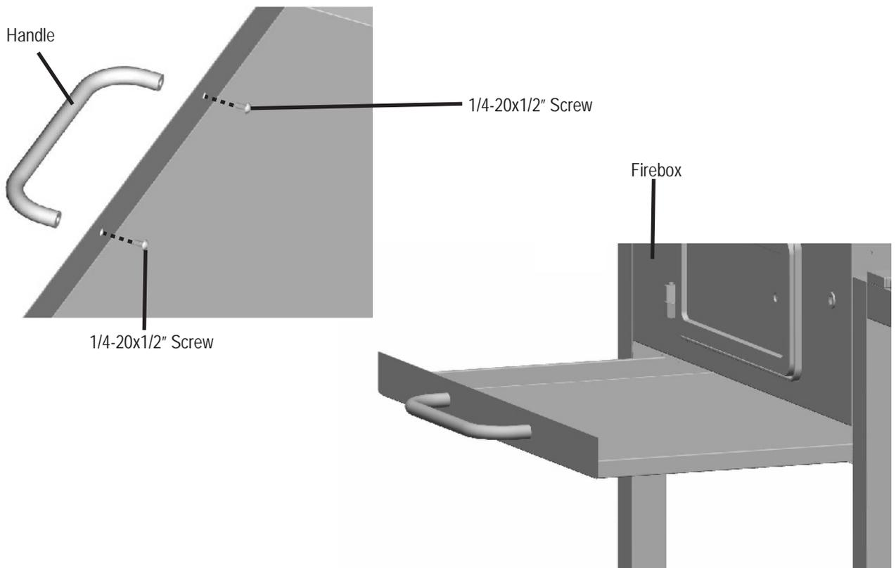
**9** Attach **Lid Handle** and **Handle Seats** to the **Lid** using (2) 1/4-20x1/2" **Screws**.
