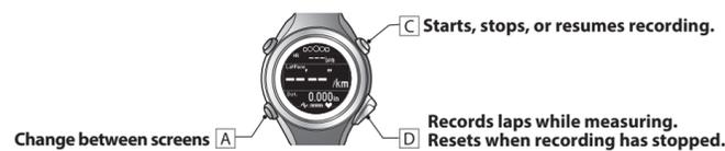
1. Press **C** on the measurement screen to start measuring.
