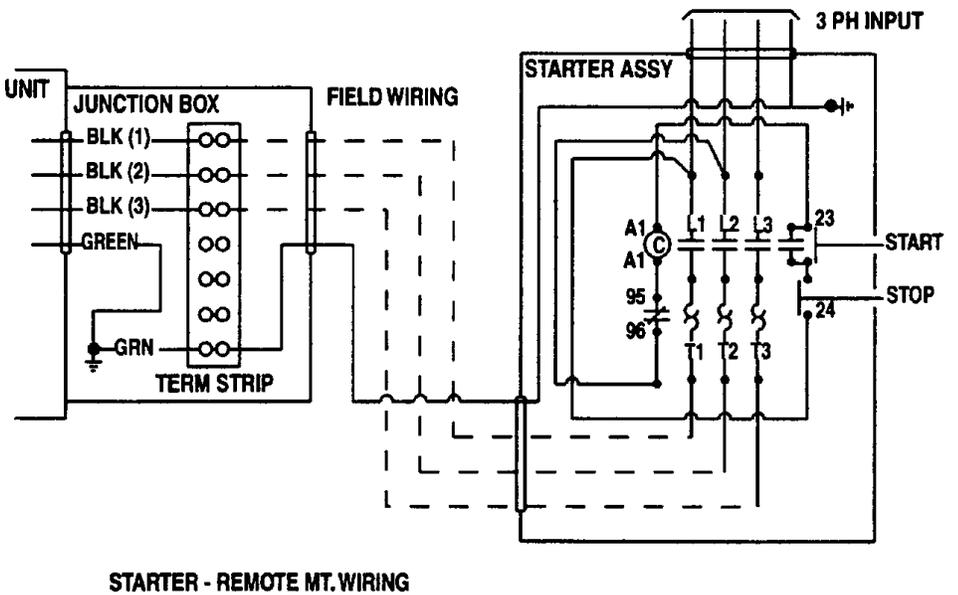
Figure 6A – Motor Wiring Diagram
