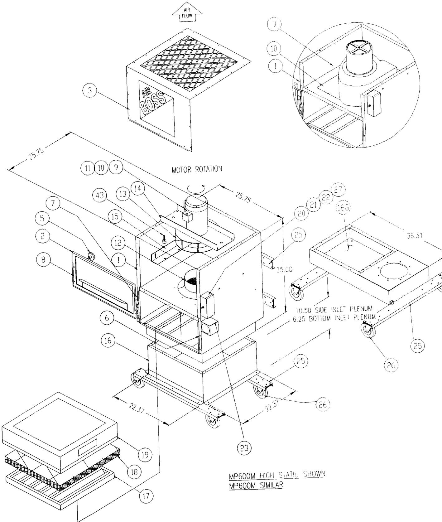
**Figure 7A – Unit Assembly Parts List**
