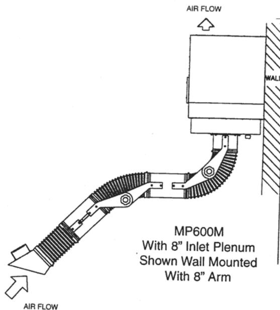
Figure 4 - MP 600M Inlet Plenum and Stand Options
