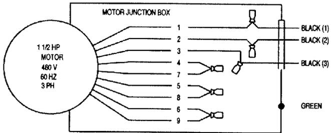
The MP600M is wired directly from the power source with 20 amps minimum, service utilizing 3 wire grounded cable, (115-208-230-460-575/60/3) for single 208-230/60/1, phase service and 4 wire grounded cable for 3 phase service, routed through appropriate conduit (See figure 5 wiring diagram). All wiring must be connected in accordance with local electrical codes.
