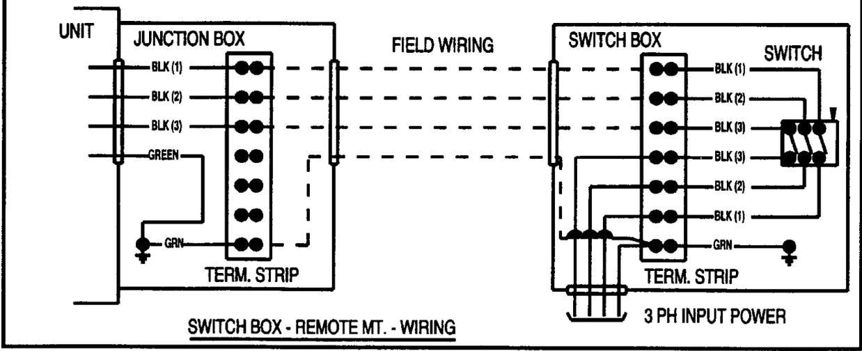
SWITCH BOX - REMOTE MT. - WIRING
