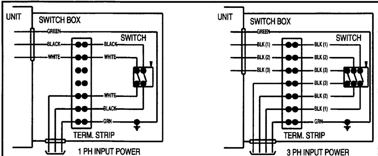
SWITCH BOX - UNIT MT. - WIRING
