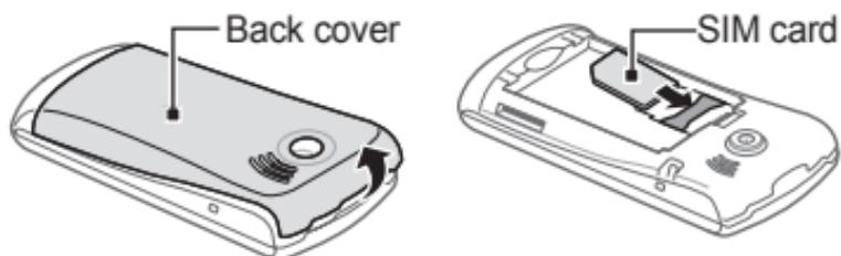
2. Insert the battery and replace the back cover.
