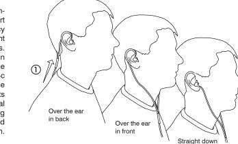
Tighten the cable and take up slack by raising the cable sleeve (1).
