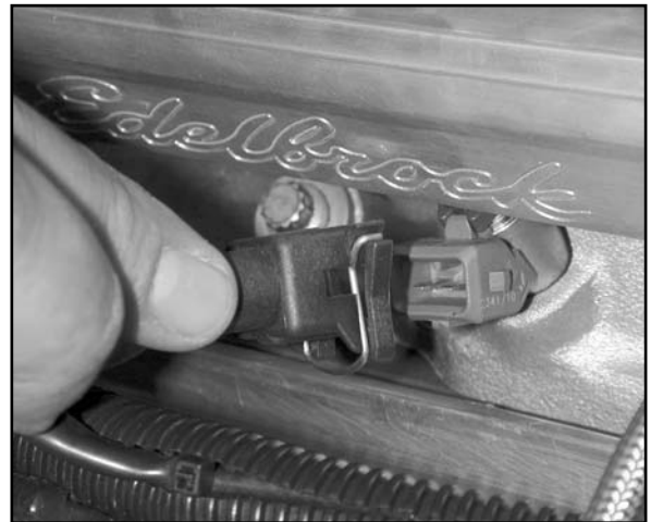
Only the fuel injector connectors are identical, but they are placed in logical sequence. Refer to the diagram when installing the harness connectors to the fuel injectors.
