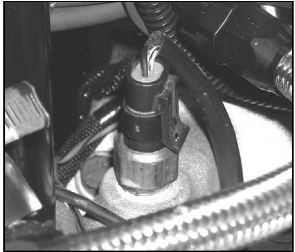
The Coolant Temperature sensor attaches to the main harness.
