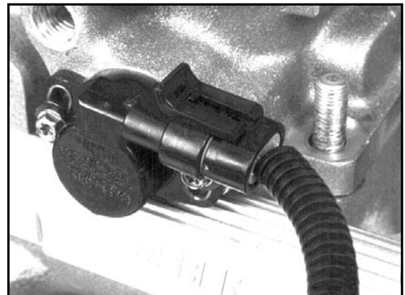
The Throttle Position sensor attaches to the main harness .
