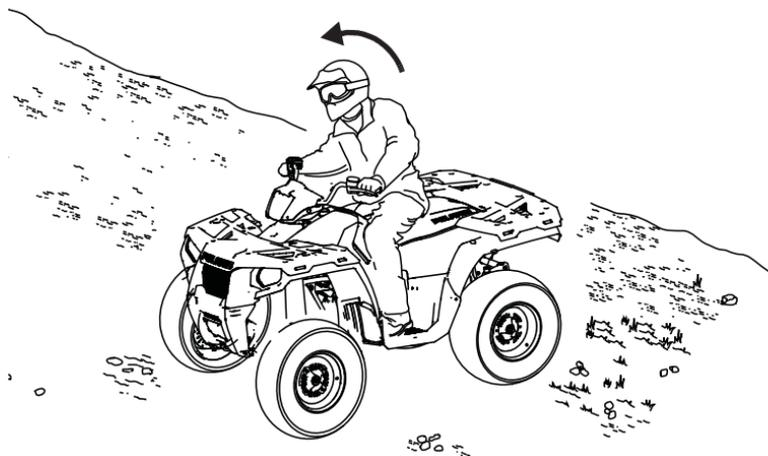
Driving on a sidehill is not recommended. Improper procedure could cause loss of control or overturn. Avoid crossing the side of any hill unless absolutely necessary.
