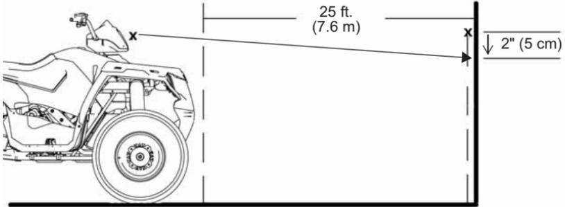
1. Position the vehicle on a level surface with the headlight approximately 25 ft. (7.6 m) from a wall. Place the transmission in PARK.
