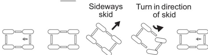
Whenever riding on slippery surfaces such as wet trails or loose gravel, or during freezing weather, follow these precautions:
