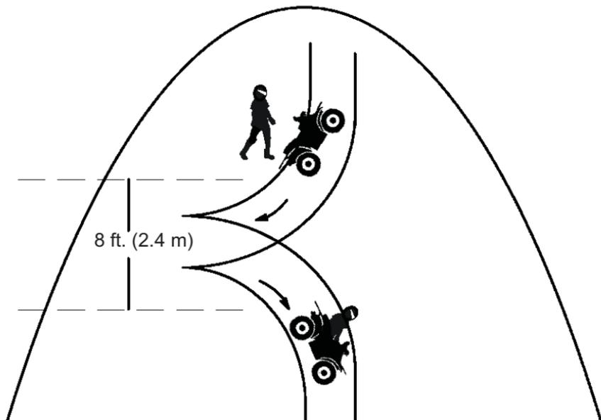
1. Stop and lock the parking brake while keeping body weight uphill.
