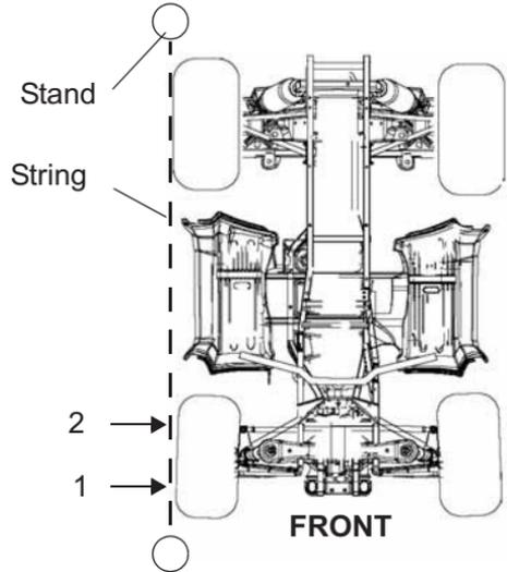
The rear measurement should be 1/16"-1/8" (2-3 mm) more than the front measurement on each side of the vehicle to obtain the recommended 1/8" to 1/4" (3-6 mm) toe out alignment.
