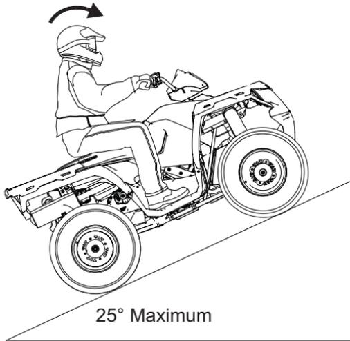
Braking and handling are greatly affected when operating in hilly terrain. Improper procedure could cause loss of control or overturn. Whenever traveling uphill, follow these precautions:
