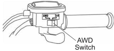
When in AWD, the demand drive unit will automatically engage any time the rear wheels lose traction. When the rear wheels regain traction, the demand drive unit will automatically disengage.
