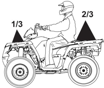
When operating over rough or hilly terrain, reduce speed and cargo weight to maintain stable driving conditions.
