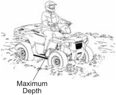
**NOTICE:** Major engine damage can result if the vehicle is not thoroughly inspected after operation in water. Perform the services outlined in the maintenance chart. See page 62. The following areas need special attention: engine oil, transmission oil, demand drive fluid, rear gearcase oil, and all grease fittings.
