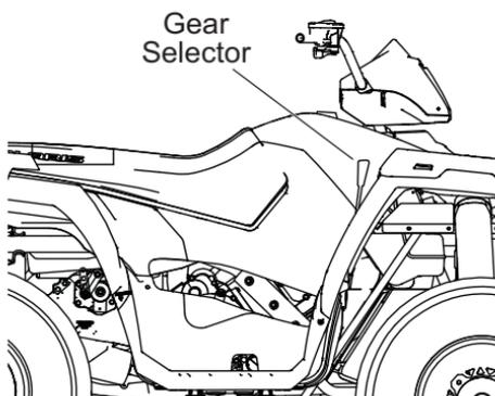
**NOTICE:** Shifting gears with the engine speed above idle or while the vehicle is moving could cause transmission damage.
