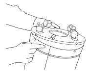
**Step 10** Replace the base, making sure the arrow on the gold sticker lines up with unit's rear seam.
