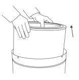
**STEP 6** Then, **remove the HEPA filter** with the same technique.
