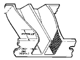
Figure 1 - Intake Manifold to Cylinder Head Port Match
