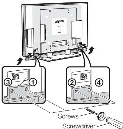
Insert and tighten the 4 screws with the screwdriver (supplied with the product) in the order of ①, ②, ③ and ④.
