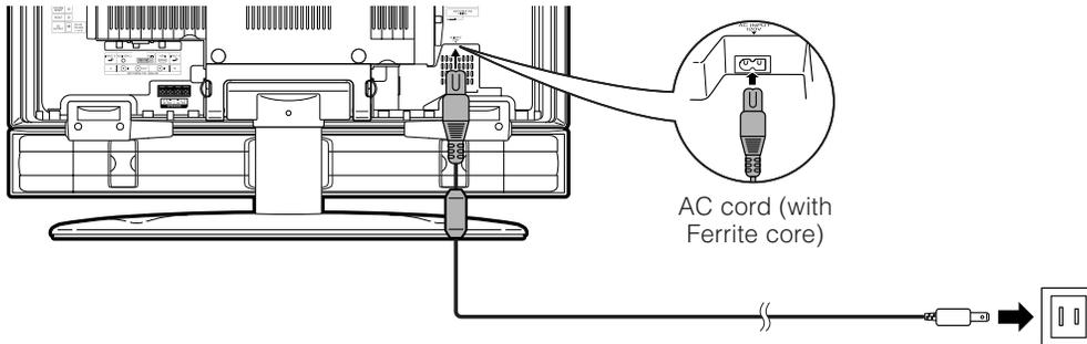
Put the Ferrite core in the space as shown in the figure. If the AC cord is not put in properly, the terminal cover may not close.
