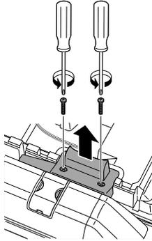
Unfasten the screw used to secure the speaker bracket.
