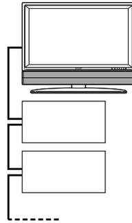
When 3 or more D-VHS decks are connected, branch connection can be used. With branch connections, up to 62 D-VHS decks can be connected.
