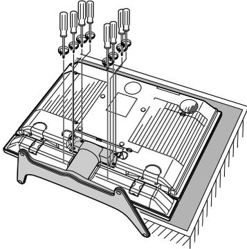
Unfasten the four screws used to secure the stand in place.
