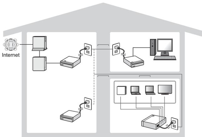
Up to four devices can be connected to the HN-VA400U adapter.
