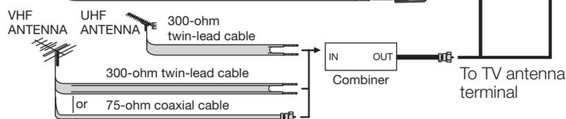
1. A 75-ohm system is generally a round cable with F-type connector that can easily be attached to a terminal without tools.
