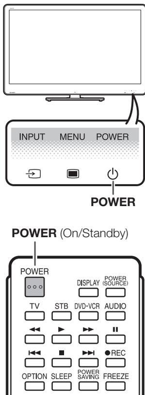
Press **POWER** on the TV or on the remote control unit to turn the power on.
