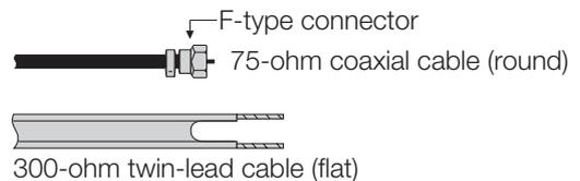
**NOTICE** F-type connector should be finger-tightened only.
