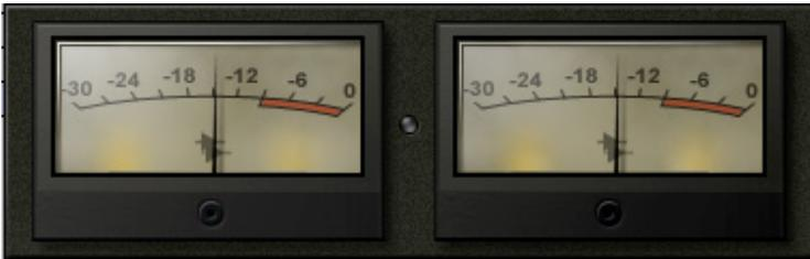
The API 560's meters display output level in dBFS. The Clip LED, located between the two meters, lights up when output signal exceeds 0dBFS.
