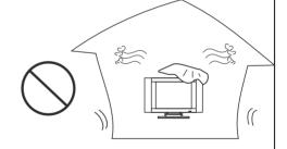
**8.Heat sources**---Do not install near any heat sources such as radiators, heat registers, stoves, or other apparatus (including amplifiers) that produce heat.
