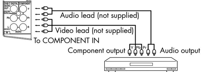
If your DVD player (or other device) has Component Video output sockets, use a suitable set of leads (RCA/Phono) to connect these to the Component Video inputs on this TV as shown - it can greatly enhance the picture quality and performance. Please remember that you will also need to connect separate leads (RCA/Phono) for the audio signals. To view this source, select the COMPONENT input mode (see page 4).
