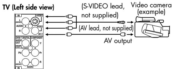
Connect the Video camera (or games console) to the TV unit using the appropriate RCA / Phono AV leads (or S-Video if applicable). Select AV2-input mode (see page 4).
